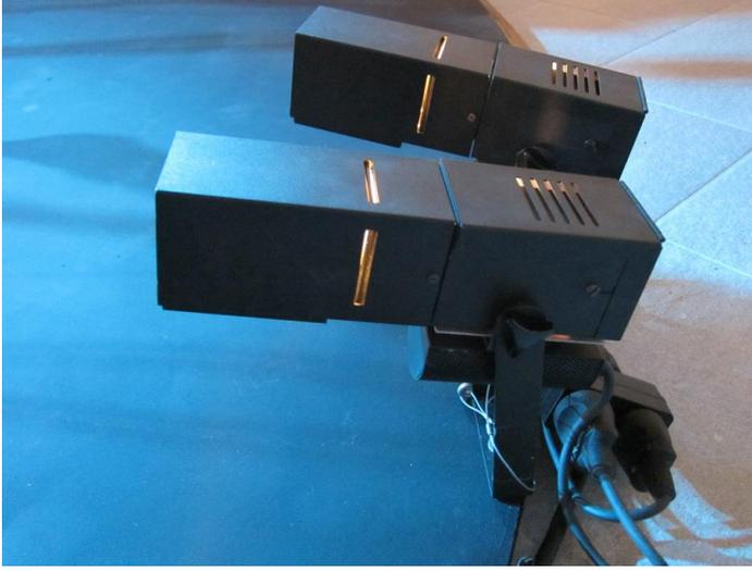
Four **Fresnel** (each 500 watts) are used to add blue colour to the legs and arms which is also on different planes so the arms and leg change colour. These fresnel are placed higher than the installation at the sides possibly on the wall about 3m high.
